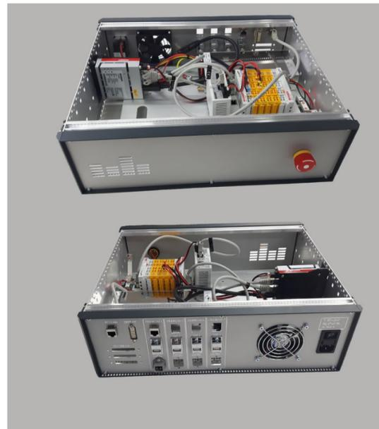
Controller for Antenna & DUT Positioners
