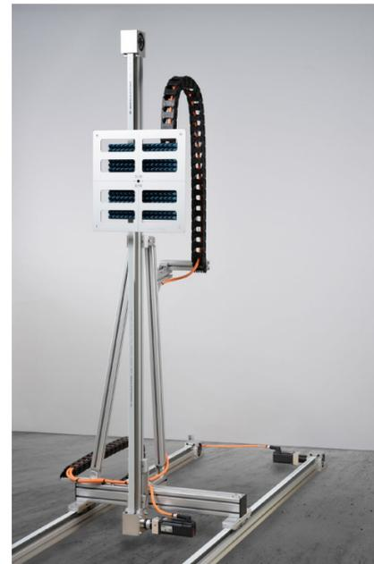
5G Antenna Positioning System for 5G Sub 6 GHz OTA Chamber
