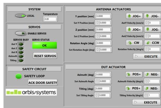
User interface for Antenna & DUT Positioners
